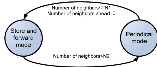
Fig. 4: Two mode model and switching mode conditions
