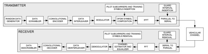
Figure 2. ITS-G5A PHY layer block diagram.
